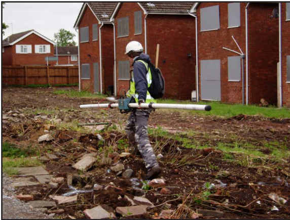
Figure 1: Acquisition of EM31 data on two former industrial sites to map foundations, underground storage tanks, voids, pipes, culverts and possible contamination plumes.
