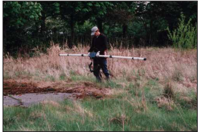
Figure 1: Acquisition of EM31 data on two former industrial sites to map foundations, underground storage tanks, voids, pipes, culverts and possible contamination plumes.
