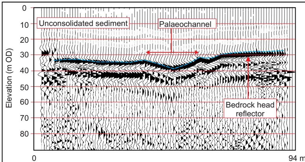
**Figure 2:** Seismic reflection section from a survey to detect sandstone bedrock beneath unconsolidated sediments in the Mersey Estuary, UK.
