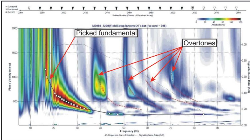
**Figure 2:** A dispersion image displayed in SurfSeis software (Kansas Geological Survey). Pre-processing to improve data interpretability has been carried out. The fundamental mode has been picked manually. Multiple overtones are also clearly identifiable.
