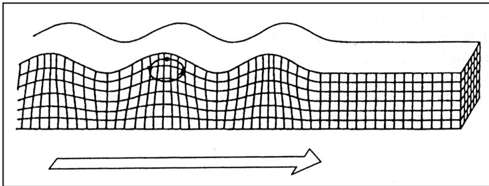
**Figure 1:** Rayleigh wave particle motion (from Bolt, 1982).
