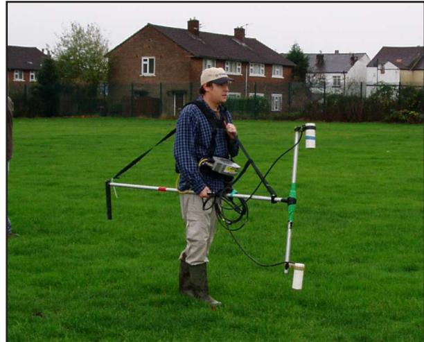
**Figure 2:** Ground-based magnetic gradiometry survey in progress.
