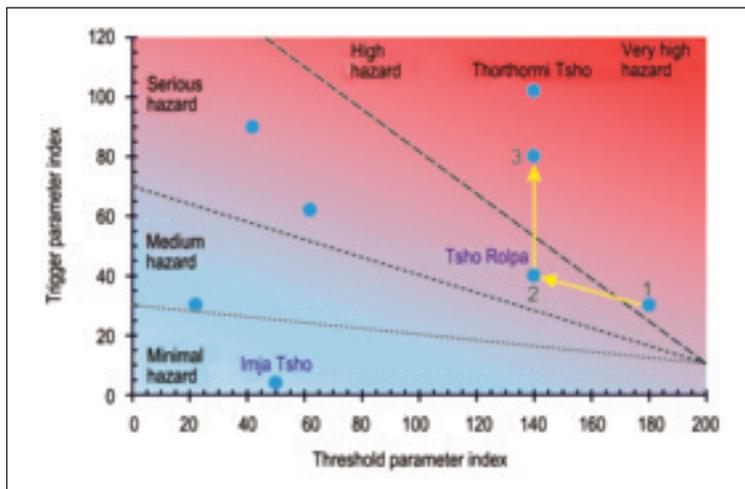
Fig. 6. Example of a Multi-Criteria Analysis hazard ranking graph. Sample scores for a number of glacial lakes are shown including Imja Tsho (Nepal) and Thorthormi Tsho (Bhutan) with three separate rankings for Tsho Rolpa, Nepal: (1) pre-interim remediation (prior to 2000); (2) post-interim remediation (2000); and (2) to (3) showing the increasing hazard associated with the growing issue of melting submerged stagnant ice until it reaches catastrophic buoyancy.
