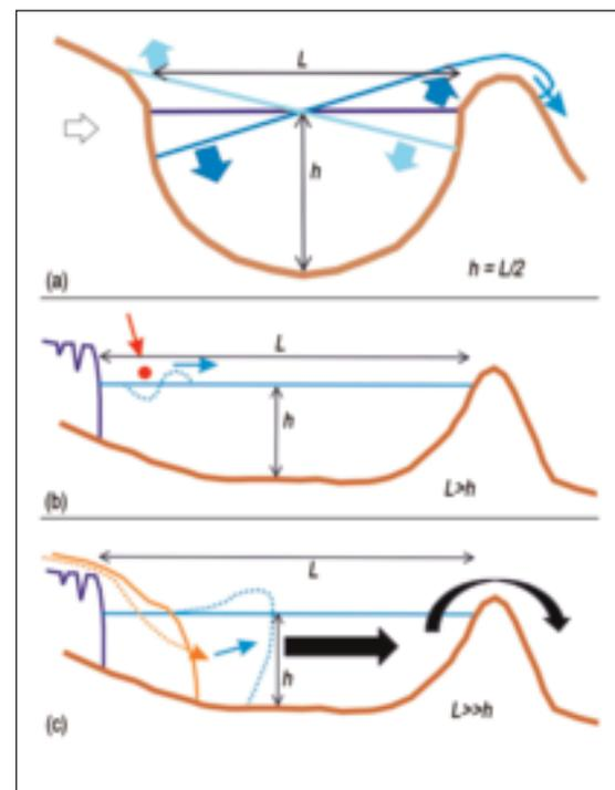
Fig. 5. Schematic illustration of how lake water behaves when influenced by an external trigger.
