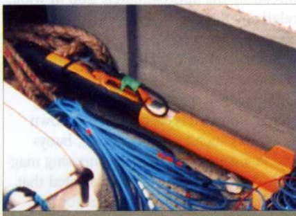
Fig. 7. Side-scan sonar tow fish used to generate a horizontal view of riverbed features and texture, enabling identification of upstanding objects
