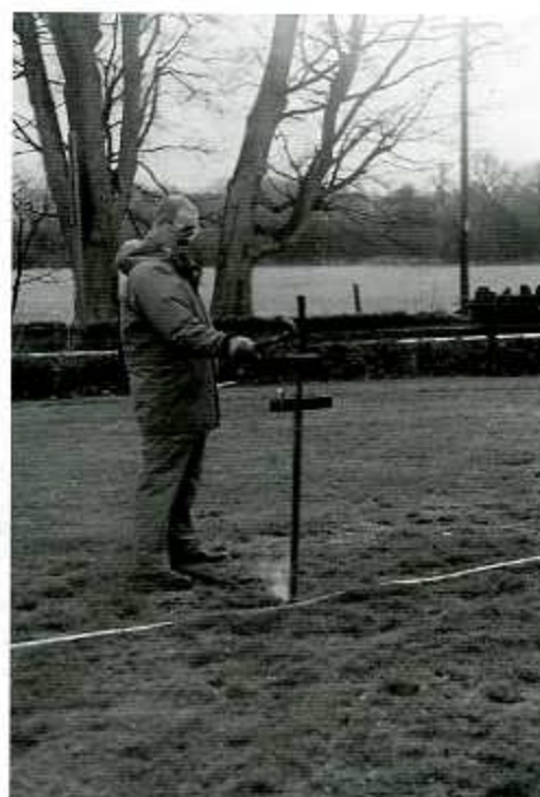
Fig. 7. Triggering the buffalo gun seismic source.
