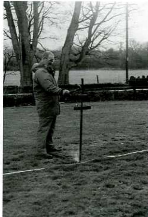
Fig. 7. Triggering the buffalo gun seismic source.
