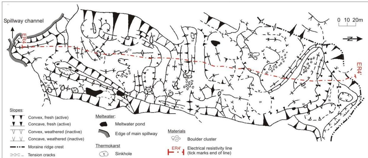
**Fig. A4.3:** Integration of various geophysical and geomorphological approaches to identify the location and thickness of buried ice, Imja Tsho, Nepal.
