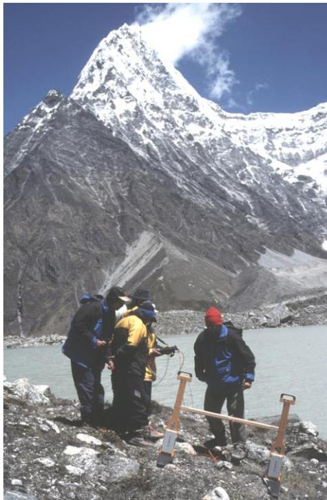
**Fig. A4.1:** Ground Penetrating Radar survey (Mala Geosciences RAMAC system) in use on moraines at Tsho Rolpa, Nepal.
