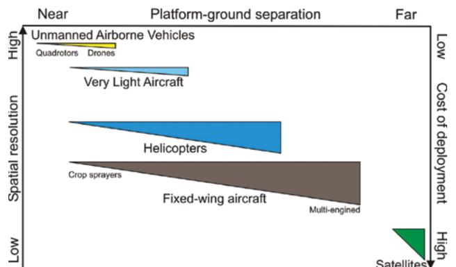
Figure 3 Schematic showing the relative ranges of spatial resolution and cost of deployment for various types of platforms for geophysical sensors.
