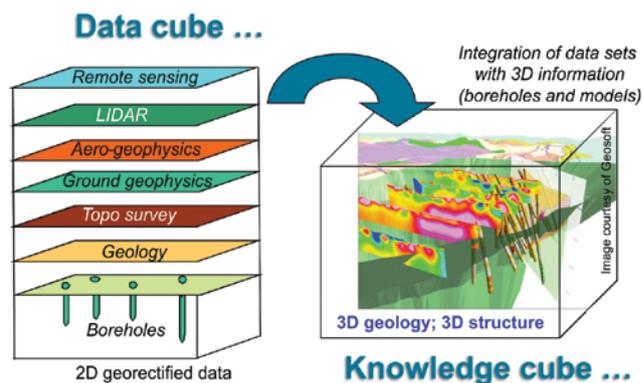
Figure 4 Inter-relationship of components within a data cube leading to a 3D ground model continuum in a knowledge cube (Reynolds, 2008).
