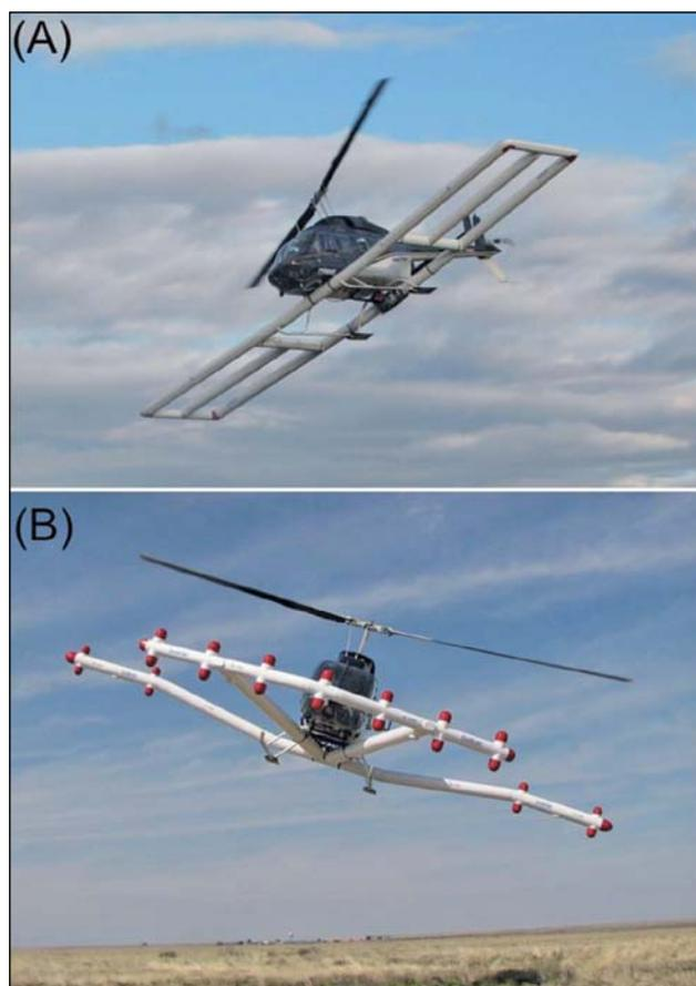
Figure 2 Airborne UXO-detection systems: (A) Battelle TEM-8 and (B) VG-22 multi-channel gradiometer. Photographs courtesy: Battelle.
