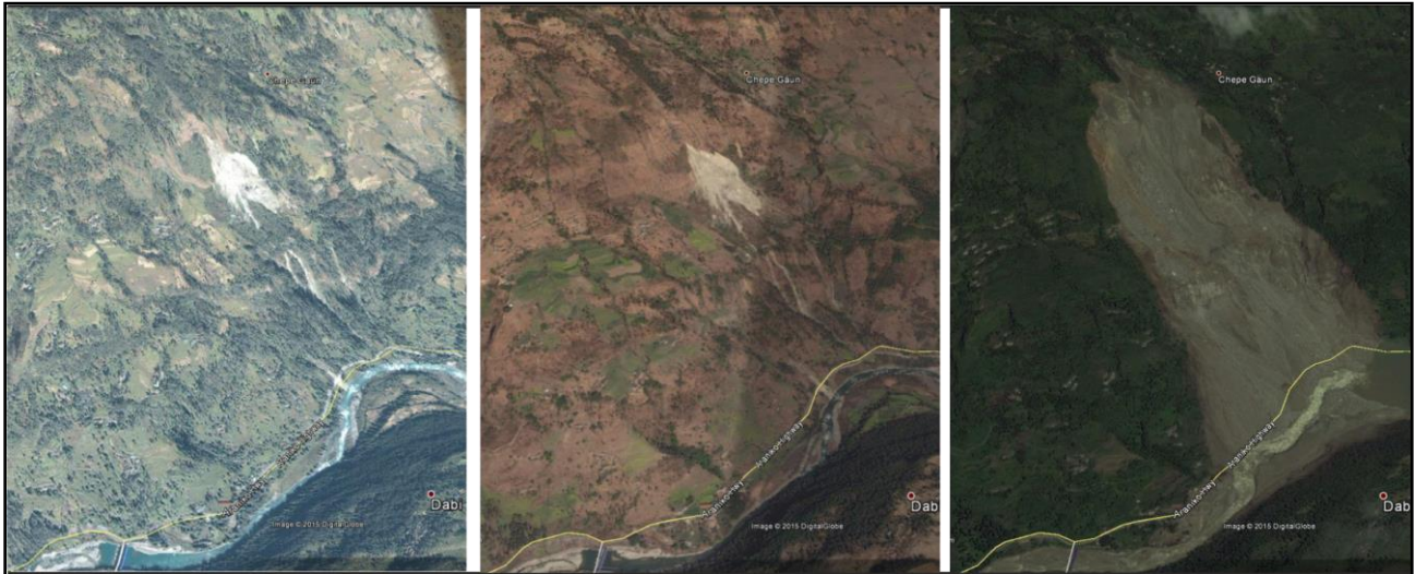
Figure 3: The development of the Sun Koshi landslide between ( left ) 31 st October 2009; ( middle ) 13 th February 2013; and ( right ) 10 th August 2014, eight days after the disaster. The location of the Sun Kosi HEP sluice gate structure can be seen across the river in the lower left of each image. (Images extracted from Google earth – © DigitalGlobe).
